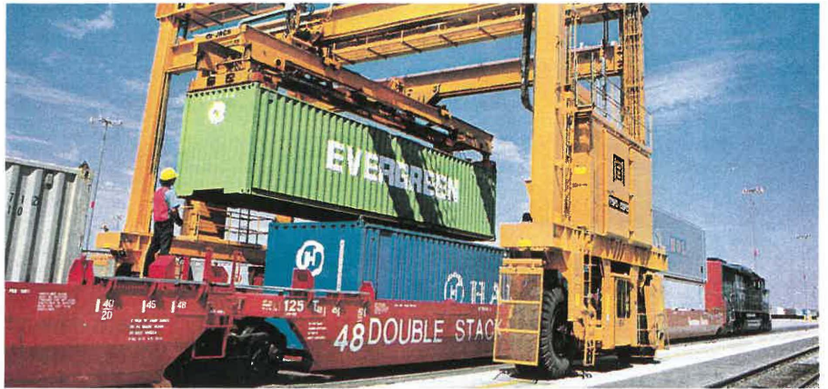
How TEUS will be loaded on trains on the Western Corridor line to the container port. 列車將使用西部走廊鐵路把貨櫃運往碼頭
